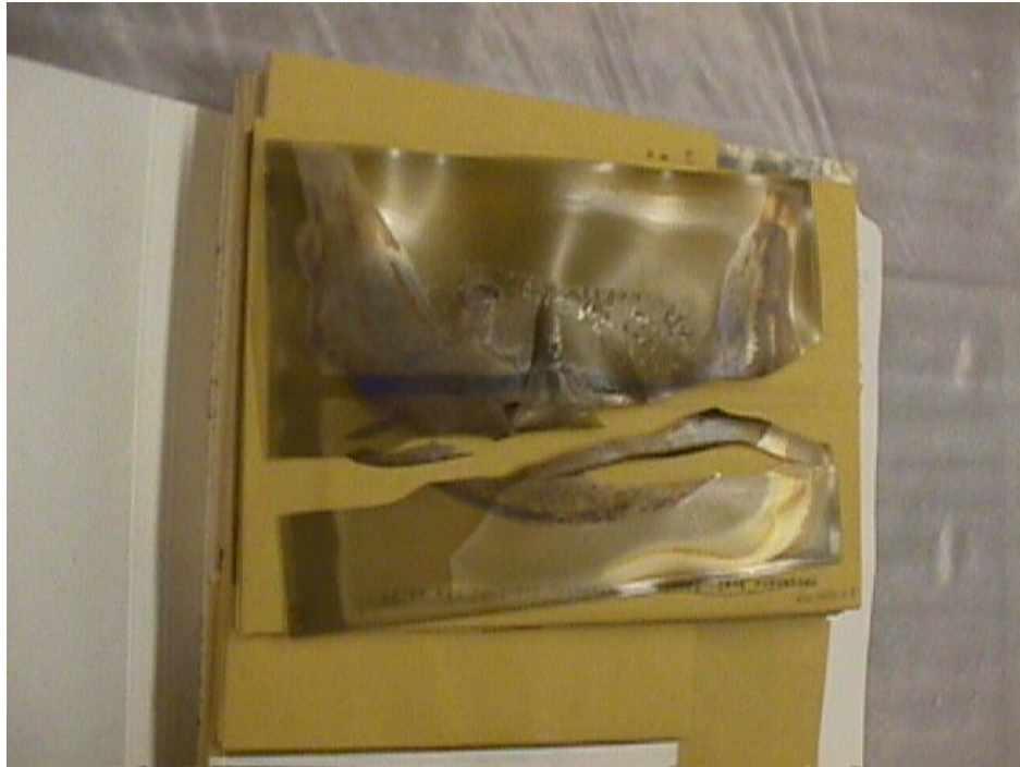
Figure 1. Cellulose nitrate negative in a state of extensive deterioration.
